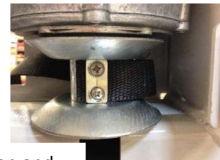
Loosen and remove roller and upper stop screw
