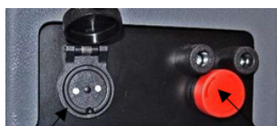
Charging connector on the lift
